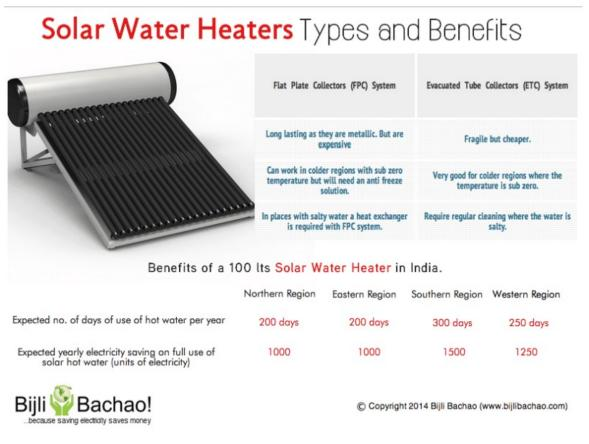
For this report, a 100-liter capacity solar water heater is considered. A 100-liter, EPC solar water require requires 20 square feet of space. The energy saving from the system is calculated a follow:
